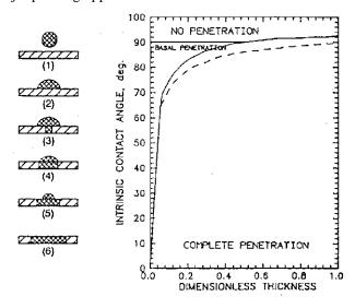
Figure 5. Theoretically calculated drop penetration modes for a thin porous medium simulating paper (Ref. 5)
