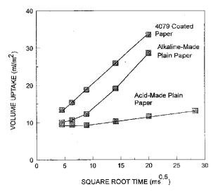
Figure 1. Penetration modes for alkaline- and acid-made papers compared to that for 4079 coated paper.
