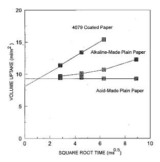
Figure 2. Short-time fiber swelling for alkaline-made paper compared to wetting delay for acid-made paper.
